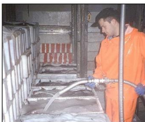
Thick Multi-Ice pumped from buffer tank at sea.
