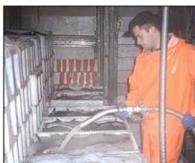
Thick Multi-Ice pumped from buffer tank at sea.
